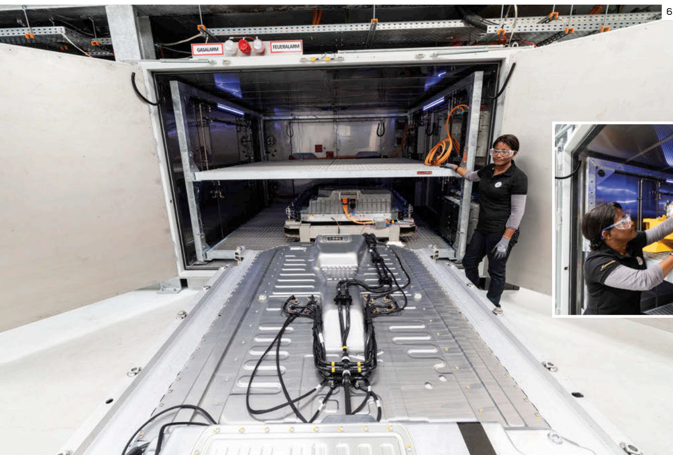
6. The Mercedes fully-electric EQC underwent extensive battery testing, including cold chamber testing to examine how cells react to extreme temperatures
